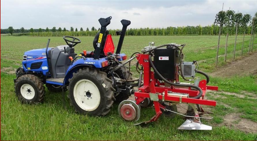
*Figure 1 Separate hydraulic system: Because of the limited hydraulic capacity of the tractor the machine is setup with its own hydraulic system. (PTO pump, tank and oil cooler).*
