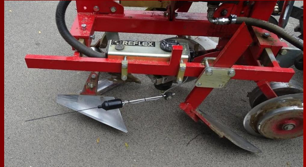
*Figure 2 Tactelec seedling sensor: Extra sensitive and light detection.*
